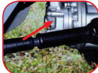
BOOST: MOTORE IDRAULICO DOPPIA VELOCITÀ - NO CE 1° 0-2 KMH / 1° VEL. 0-4 KMH 2° 0-10 KMH / 2° VEL. 0-20 KMH BOOST: HYDRAULIC MOTOR DOUBLE SPEED-NO CE 1ST 0-2 KMH / 0-4 KMH - 2ND SPEED / 0-10 KMH 0-20KMH BOOST: HYDR. MOTOR DOPPELTER GESCHWINDIGKEIT NEIN CEE. 1. 0-2 KMS / 0-4 KMS 2. GANG 0-10KMS / 0-20 KMS BOOST: MOTEUR HYDRAULIQUE DOUBLE VITESSE NO CEE. 1ERE VITESSE 0-2 KMH / 0-4 KMH - 2EME VITESSE 0-10 KMH / 0-20KMH BOOST: MOTOR HIDRAULICO DOBLE VELOCIDAD NO CEE. 1ERA VELOCIDAD 0-2 KMH / 0-4 KMH 2DA VELOCIDAD 0-10 KMH / 0-20KMH
