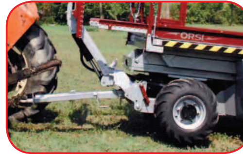
KIT SOLLEVAMENTO E TRAIKO KG 22 UPLIFTING AND TOWING KIT HEBEKIT MIT ZUGDEICHSEL KIT SOULEVEMENT ET DE REMORQUAGE KIT DE LEVANTAMIENTO Y REMOLQUE OMOLOGAZIONE STRADALE SOLO ITALIA (CROSS, COMPACT, GRANDINE)
