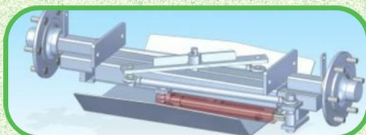
The hydraulic axle can be adjusted up to 30 cm. This helps with not only stability but with offsetting the issue of compaction across a larger area.
