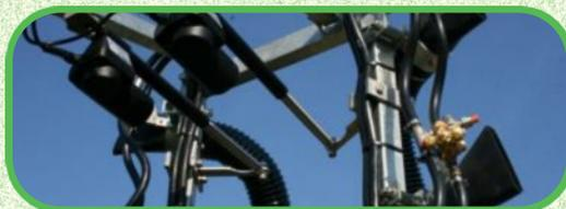
Electric air adjustment of cowlings improves liquid deposition and reduces drift.
