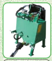
Independent PTO Hydraulic system; pump, heat exchanger, 60 L holding tank
