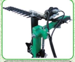
Horizontal topping bar with 90° rotation and spring loaded for safety around posts
